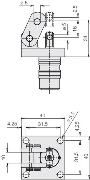
**Clamping lever with contact bolt**
