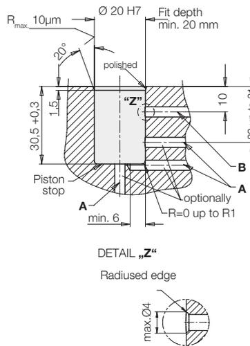
**Connecting dimensions for self-manufactured clamping levers**
